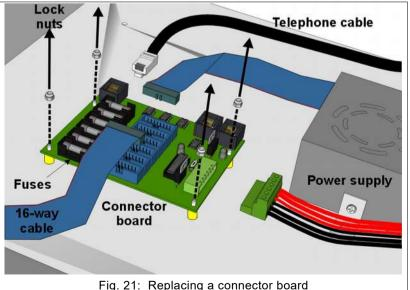
Fig. 21: Replacing a connector board
