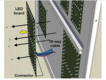
Fig. 20: Replacing a LED display board
