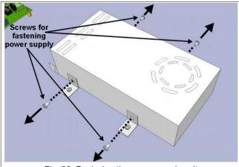
Fig. 22: Replacing the power supply unit
