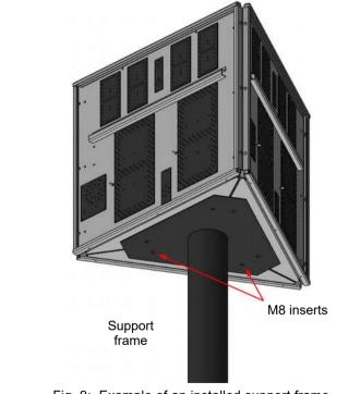
Fig. 9: Example of an installed support frame
