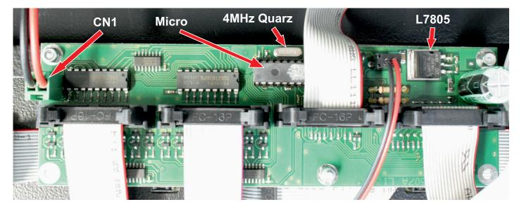
Fig.5 FAV.A507 - CPU Electronic board for PS-x
