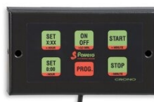
Art.334 ...Additional keyboard for CRONO and CRONO-M With cable 1,3m long. Size: 15,5x9x1,6cm. - Weight: 0.43kg.
