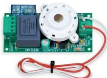
Art.A4-115 ...RADIO-SPARK-115 Interrupts the power supply of a device powered by 115Vac. Size: 10,4x5,1xH4,2cm. - Weight: 0.24kg.
