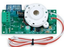
Art.A4-024c ...RADIO-SPARK-24Vdc Interrupts the power supply of a device powered by 24Vcc. Size: 10,4x5,1xH4,2cm. - Weight: 0.14kg.
