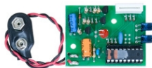
Art.0430-0360C FAV.9506B electronic board for the FIGHT-TIMER remote control Spare part for art.150-02 Size: 5x3,9cm. - Weight: 0.017kg.
